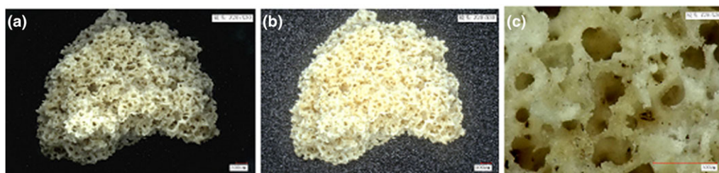
Figure 4 Observation by the 3D deep-field microscope: (a) real-time zoom lens (RZlens) imaging (magnification \times 30 ); (b) High dynamic range (HDR) function imaging, synthesizing 3D images by capturing multiple colour images at different brightness levels (magnification \times 30 ); (c) RZlens imaging (magnification \times 200 ). [Colour figure can be viewed at wileyonlinelibrary.com ]
